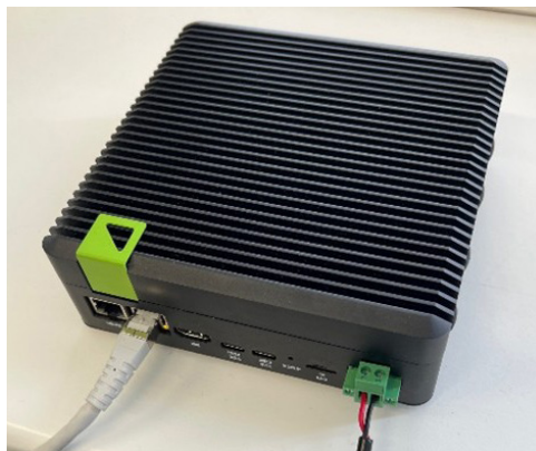
Abbildung 6: Nvidia Jetson Orin NX 16 GB Industrial (Seeed Studio reComputer Industrial J4012), passiv gekühlt. Quelle: Fraunhofer IPA/Foto: Timo Leitzitz.
